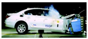
Offset crash test at 64km/h
