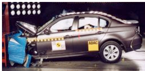
Offset crash test at 64km/h
