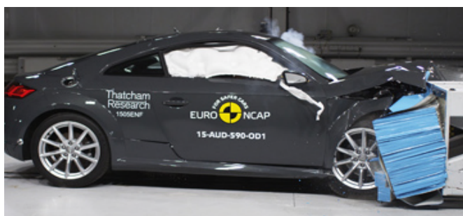
Frontal offset test at 64km/h
