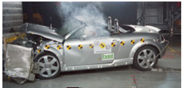
Offset crash test at 64km/h
