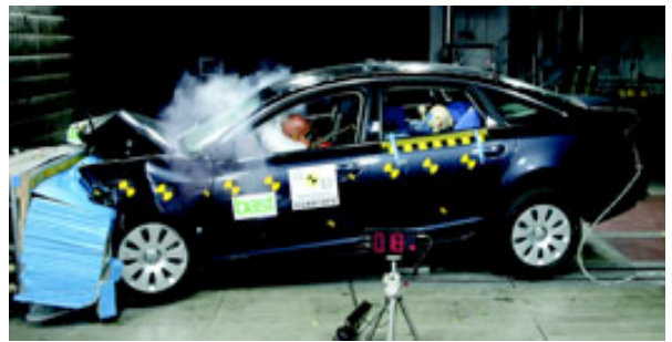
Offset crash test at 64km/h
