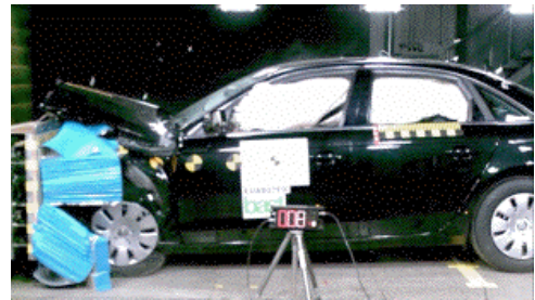
Offset crash test at 64km/h
