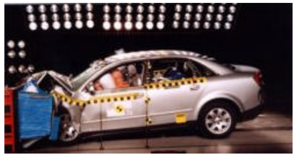
Offset crash test at 64km/h
