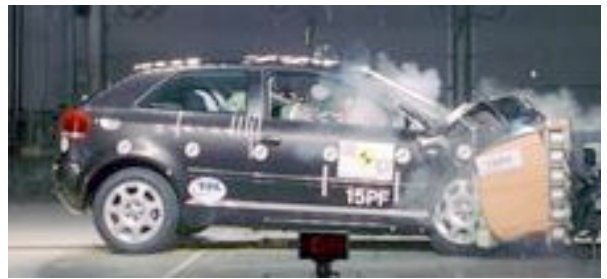
Offset crash test at 64km/h
