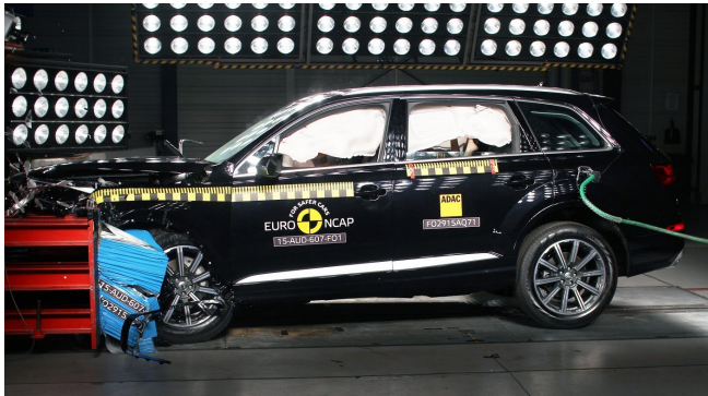
Frontal offset test at 64km/h
