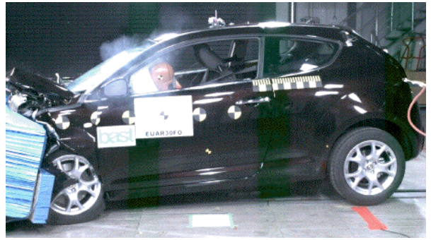
Offset crash test at 64km/h
