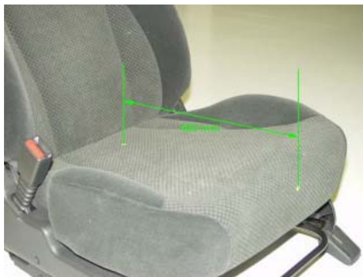
Figure 5: Measurement of cushion angle
