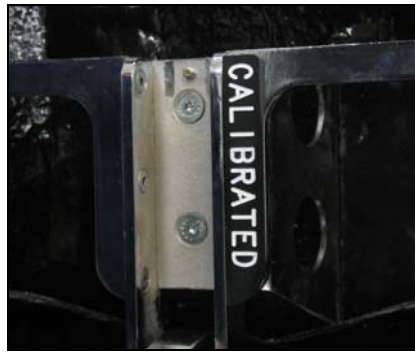
Figure 10. Calibrated Torso angle measurement surface block attached to trunk of weight hanger arm.
