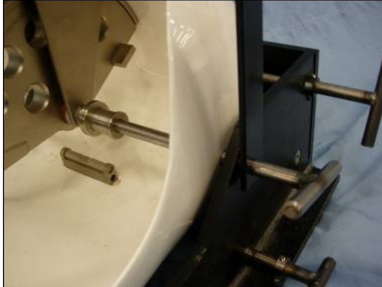
Figure 3. H-Point locator bars installed through vertical support rods, jig side and H-PM H-Point location.
